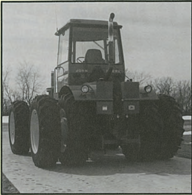
Rear view of 830 Special, showing twin fuel tanks.
