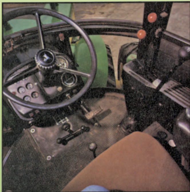
Inside of the cab with dual gear shift levers on floor. The hand clutch is to the right of seat.
